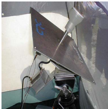
Figure 4b: Briefcase terminal with 44-cm reflectarray
