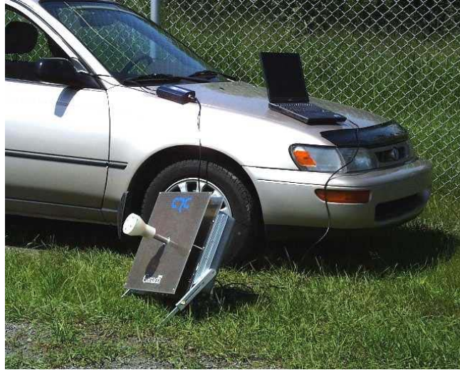
Figure 6: Ka-Pak terminal – Typical setup.
