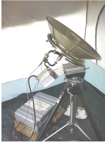
Figure 4a: Briefcase terminal with 44-cm parabolic reflector
